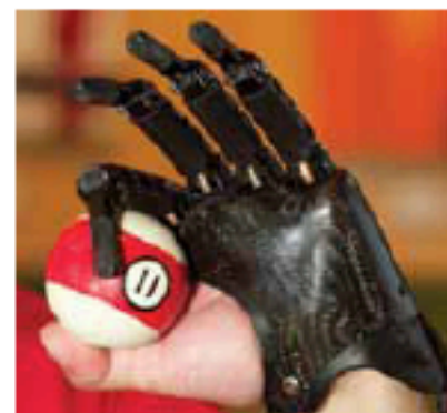
Innovative prosthesis technology Individually articulating electronic fingers are a break-through in prosthetic technology. PHOTO: COURTESY OF ADVANCED ARM DYNAMICS
